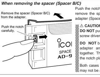
Push the notch carefully with your finger to remove the spacer (Spacer B/C) from the adapter (Spacer A).
